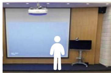
Meanwhile, when there is another presenter appears within the current camera view and then detected by the camera, the camera will be triggered to the pre-configured preset position.
